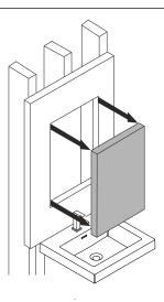
Cut the marked perimeter with suitable tool.
