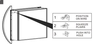
Fix the wire with terminals as shown diagram
