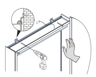
Top mounting brackets must be attached to furring strip/channel or wall studs.
