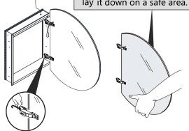
While supporting the door release (the lever under the hinge arm), slide the door off the frame.
