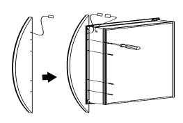
Door with wire pass through the wire hole, Other holes are aligned, and tighten the screw with a screwdriver
