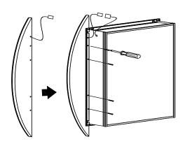
Door with wire pass through the wire hole, Other holes are aligned, and tighten the screw with a screwdriver
