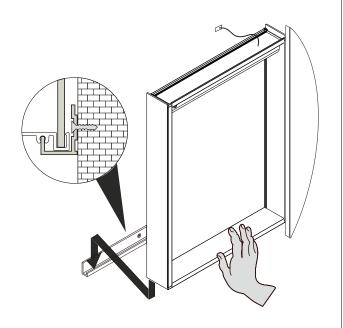
With assistance, to rest the cabinet on the mounting bracket and hold in place.
