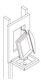
Connect electrical wires before inserting the cabinet into the opening.
