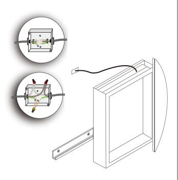
Connect the wire to Junction Box inside the wall.
