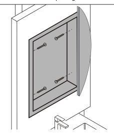
Affix using hardware screws into the studs.
