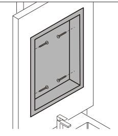
Affix using hardware screws into the studs.
