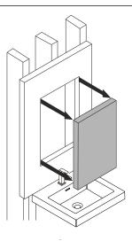
Cut the marked perimeter with suitable tool.
