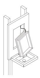
Connect electrical wires before inserting the cabinet into the opening.
