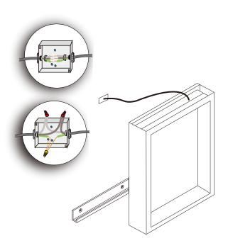
Connect the wire to Junction Box inside the wall.
