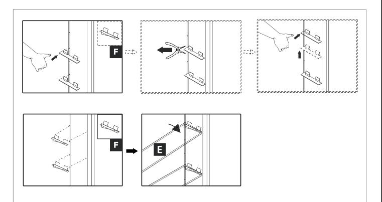
1.Insert clear snap in shelf clips (F) into holes on the sides of the cabinet.
