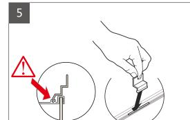
Insert top mounting bracket into the top of the cabinet.
