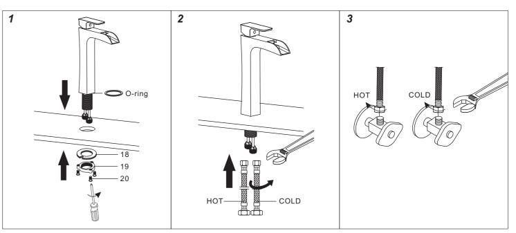
to the base of faucet. Fix the 3 screws #20 by screwdriver.
