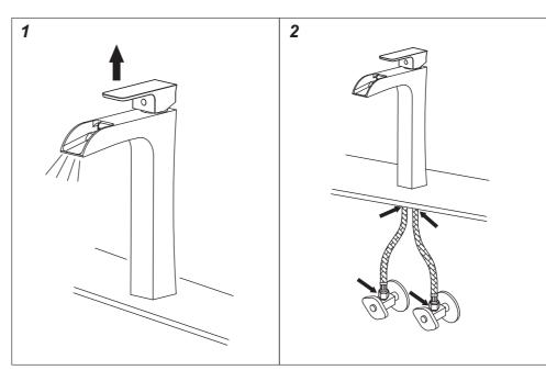
1. Turn the faucet handle all the way on, turn on hot and cold water supply and flush water lines for one minute. 2. Check all connections at arrows for leaks, re-tighten it if necessary. BUT DON'T OVERTIGHTEN
